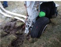
We attempted to move the E-2B in March 2016, but the ground was so saturated that the aircraft's left main landing gear sunk into the mud. Getting the 30,000 lb. aircraft free again would take some work. Charlie A. reached out to the community for some assistance.
